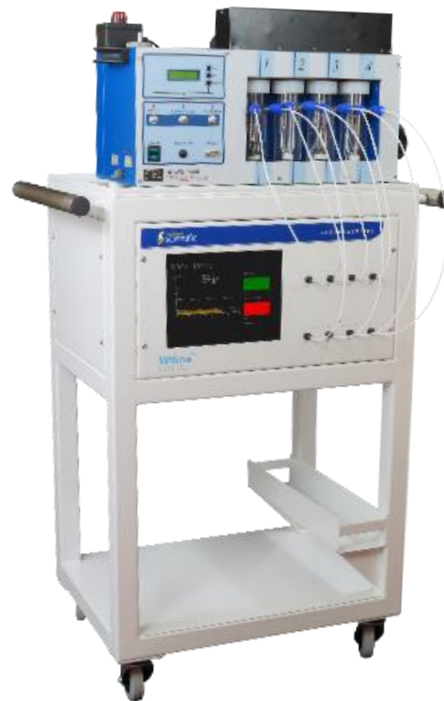
WILMA-Bubbler – On-line air/water monitoring system
